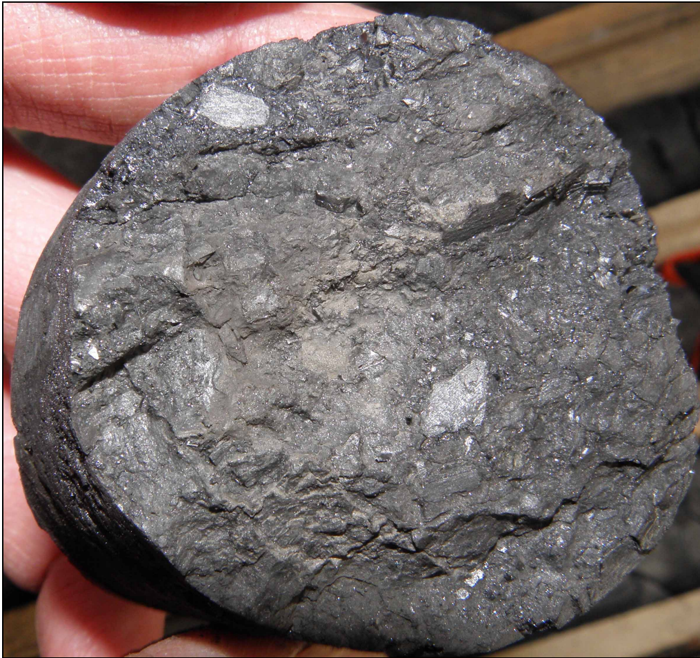
Photo 6: Coal bed at 270.2m, approximately 0.3cm. Looking at the bedding plane, the shiny pieces are carbonaceous material (coal), while the dull parts are probably mud (ash). The coal appears to be fragmental which could indicate that it has been transported into the sedimentary basin.
